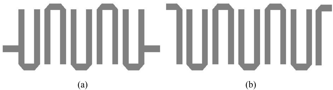
Fig. 6: (a) tapped line input 5-pole Hairpin Filter. (b) coupled line input 5-pole Hairpin Filter.
