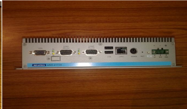
Fig.:-2 Rear view of Embedded CPU
