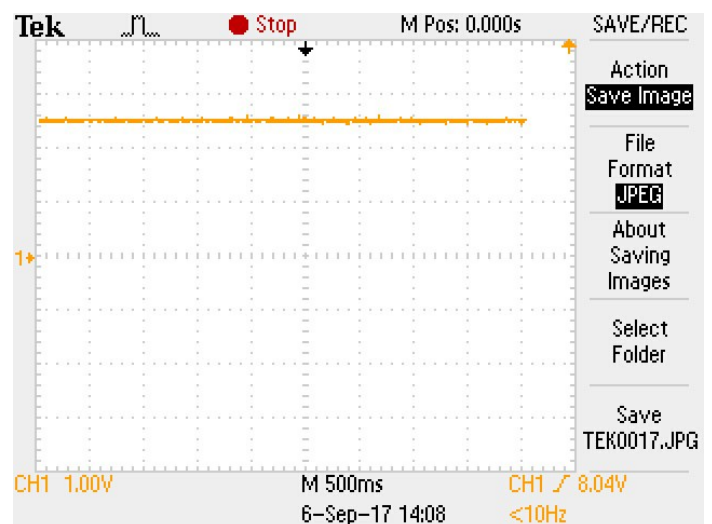
Fig 11 : Voltage level at inverting output
