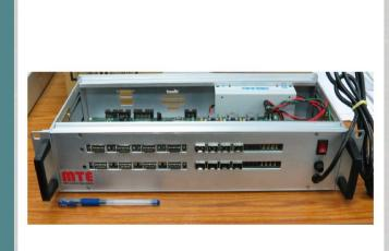
This unit converts the 10Gbps ethernet outputs on ROACH to SFP+ standard for use with network switches – developed in collaboration with MTE, Pune.
