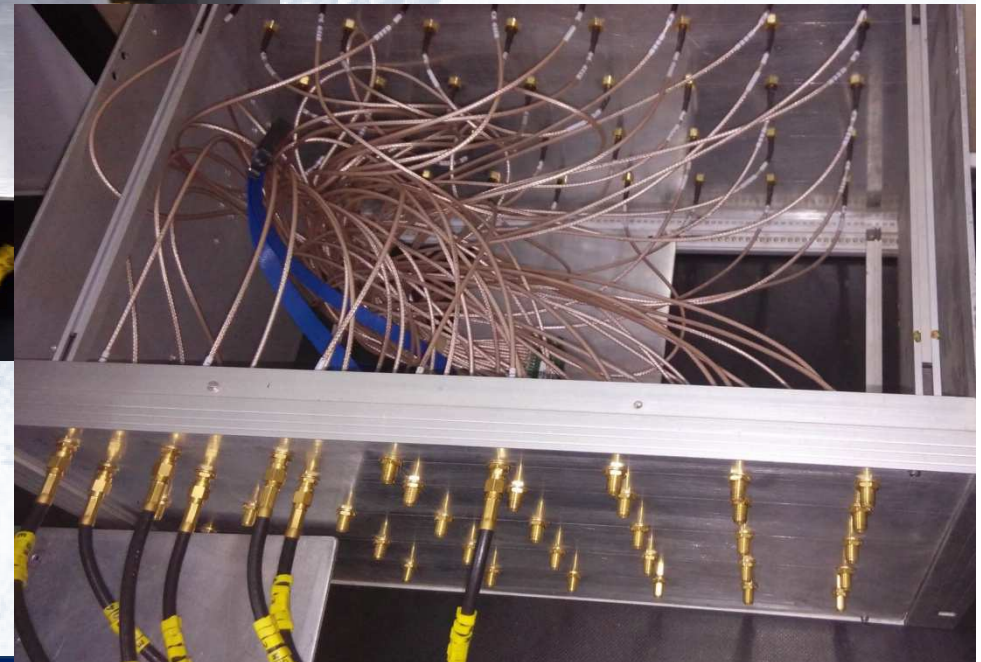
64-channel ADC connected with the ROACH-1 board (above)
