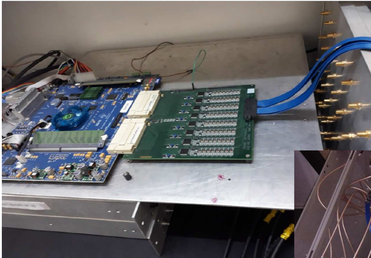
64-channel ADC connected with the ROACH-1 board (above)
