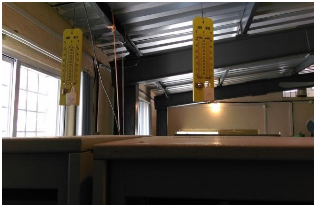
Figure 23: Setup for monitoring FPA Racks temperature
