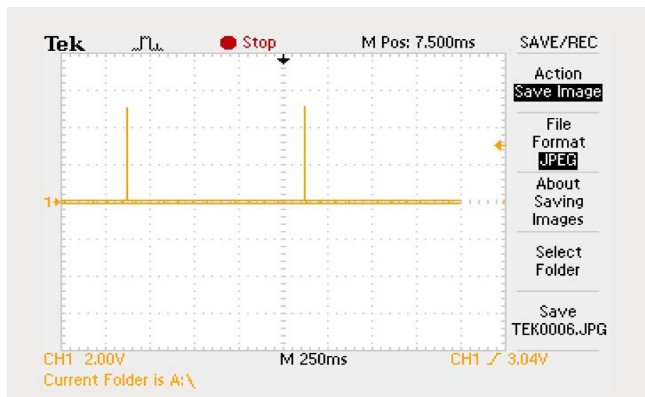
Figure17: Plot for 1 PPS signal from Rubidium (Digital Processing Board subrack1).
