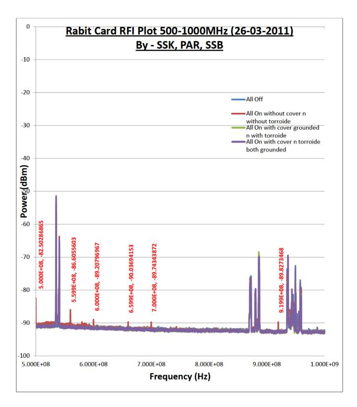
**Remark**: After power ON condition of RABIT CARD 500-1000 MHz Frequency band shows discrete lines but it is in some specific pattern which are equally spaced of 40 MHz. There are two sub bands which having 60 MHz space in between them.
