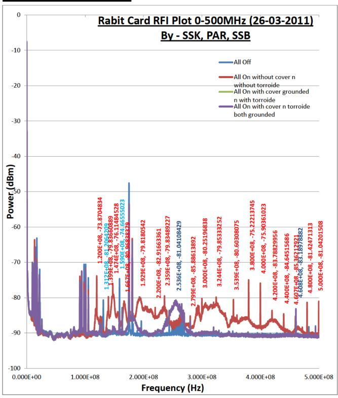
**Remark**: After power ON condition of RABIT CARD 0-500MHz Frequency Band shows so many discrete lines most of them are equally spaced of 20MHz.
