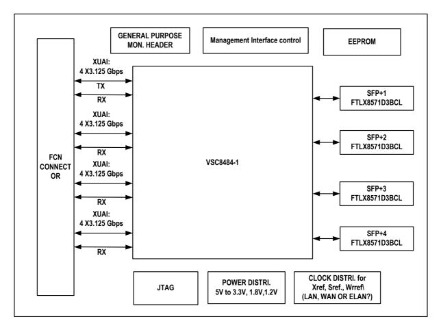
PHY chip on the adapter board requires low jitter clock oscillator, regulated power supply, EEPROM and reset control circuit for its functioning. The EEPROM has to be programmed using the hex file available from the vendor. The board also needs header connectors for I2C, MDIO and GPIO interfaces.
