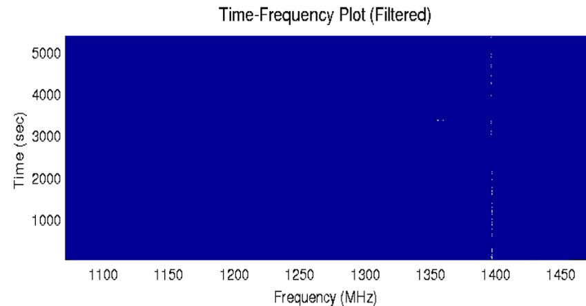
Narrowband RFI filtering on GWB-3 recorded data (L-band)
