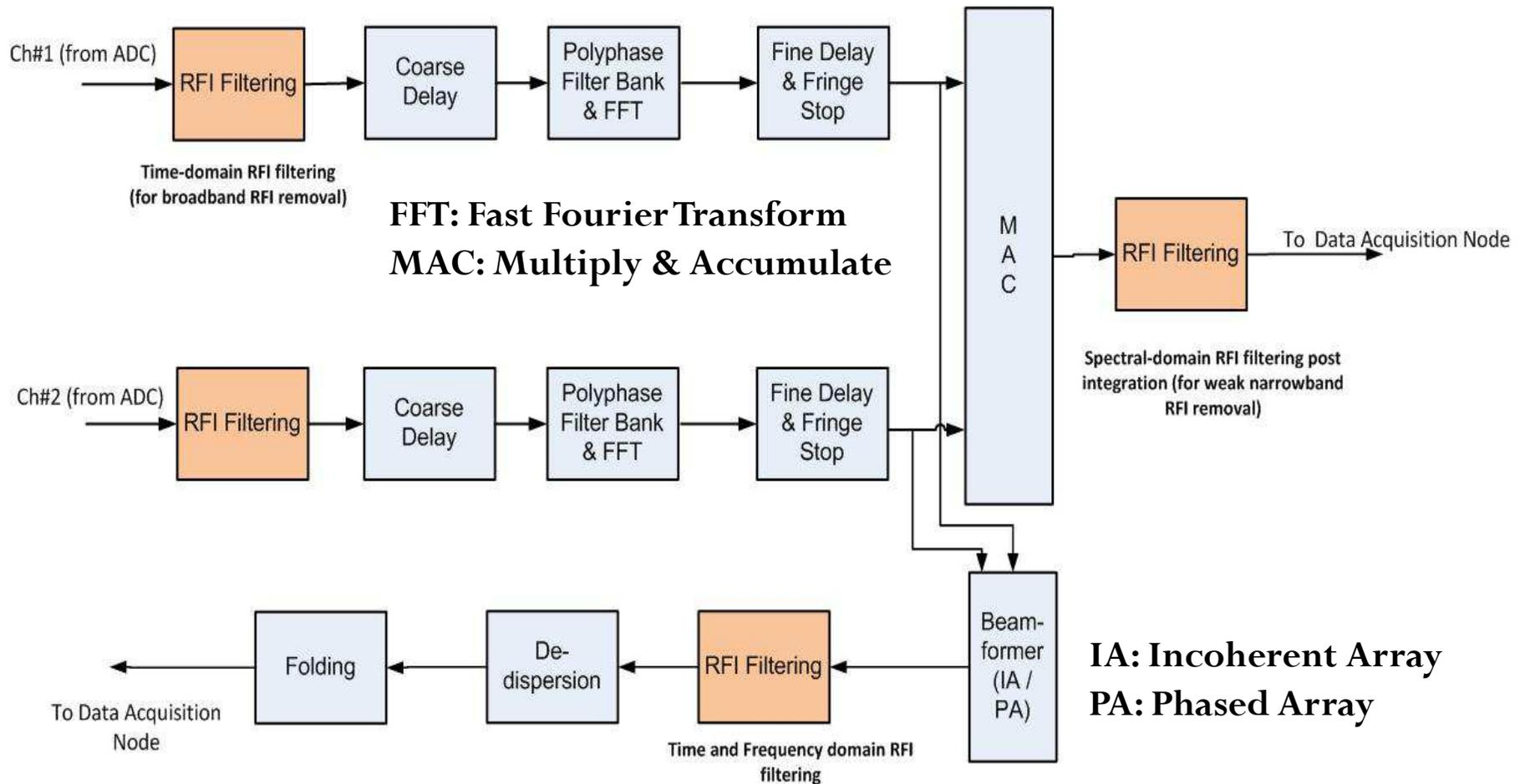
❑ Requires implementation at multiple locations in the processing chain to remove diverse types of RFI
