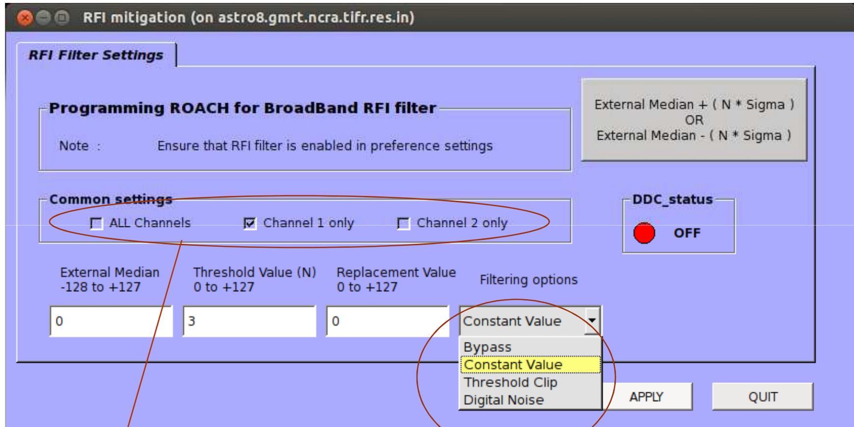
Can filter one or both polarizations
