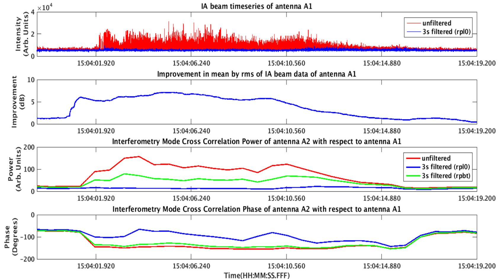
Beam and correlator data of a spectral channel showing filtering at  $3\sigma$  threshold – replacement with zero and threshold
