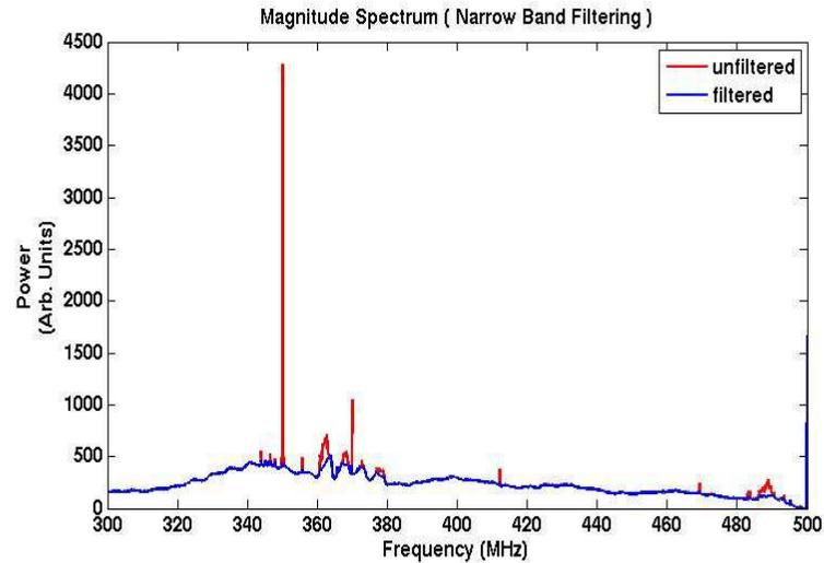
Narrowband filtering removes strong lines in the spectrum
