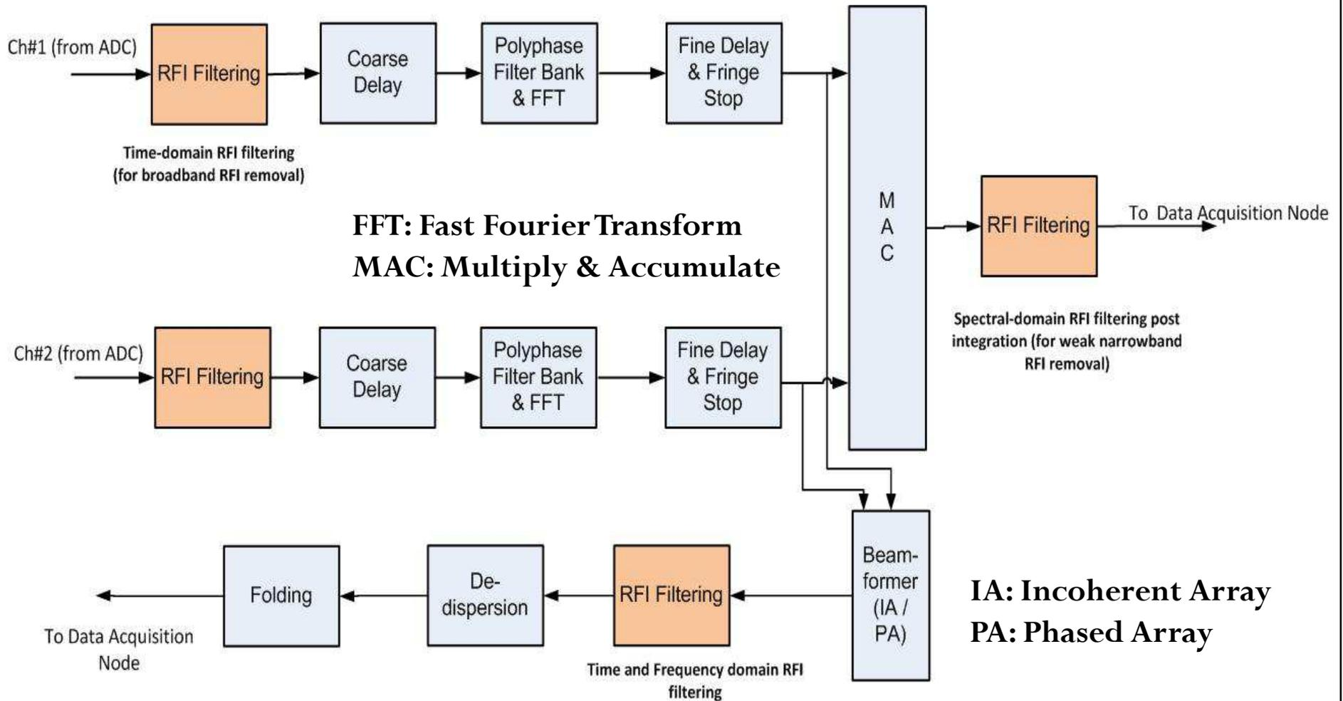
Real-time Narrowband RFI Mitigation is carried out post-integration at 0.671s integration on visibilities
