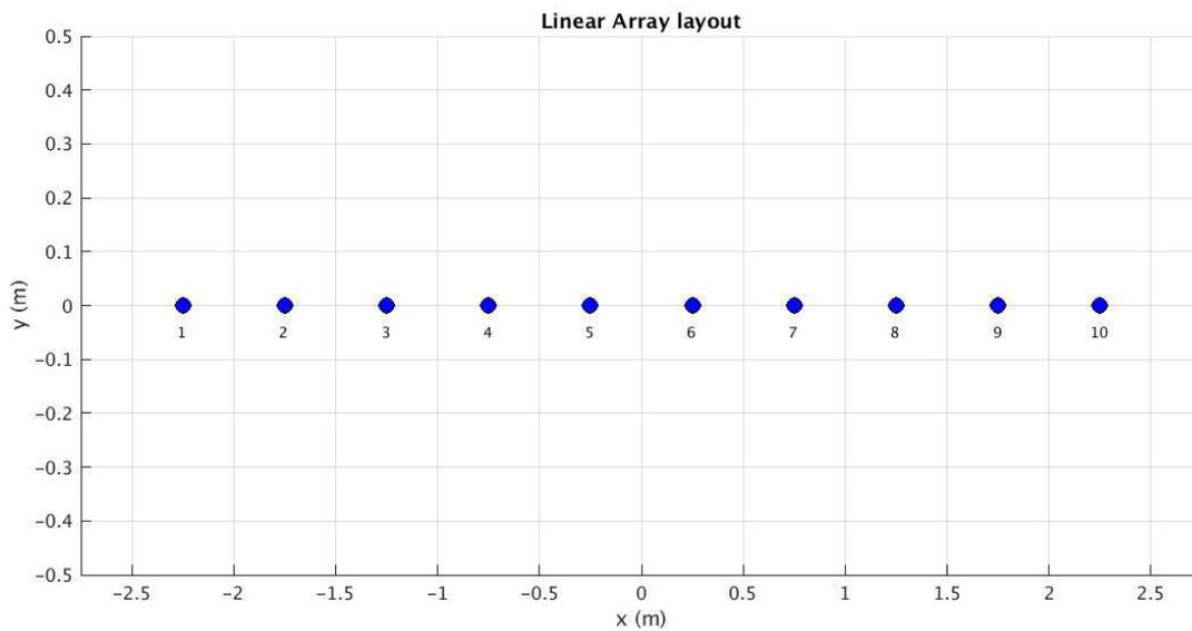
Image 22: Linear array layout for 10 dipole elements
