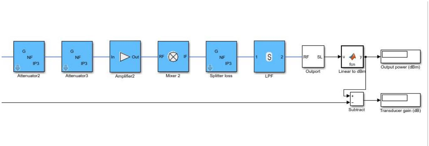
Image 39: Screenshot showing receiver chain exported to simulink environment (Second half)
