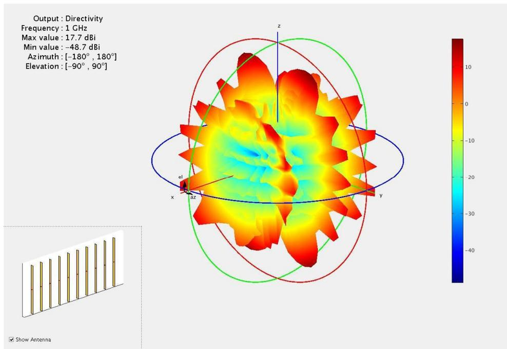
Image 24: Radiation Pattern of the linear Array
