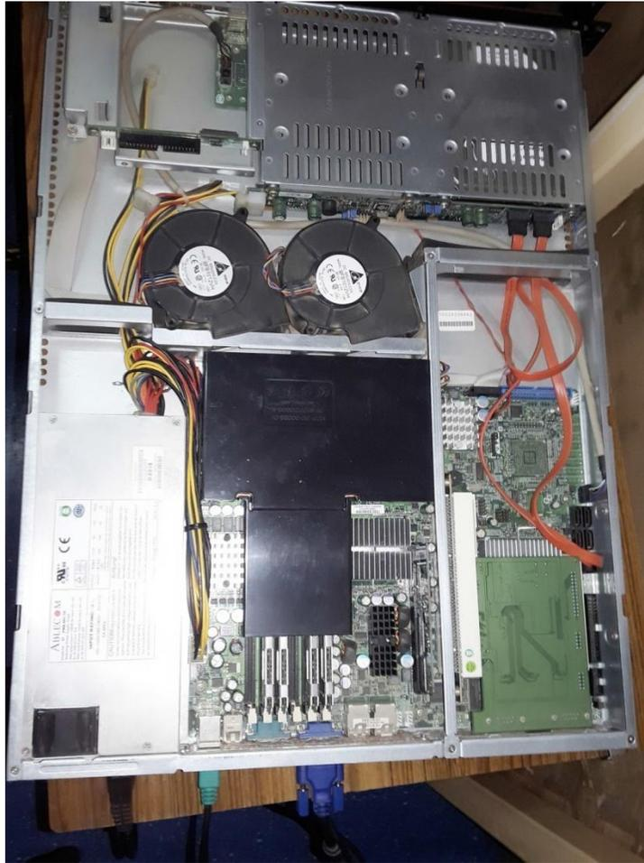
Image 12 : Local Control Unit (PC) after dismantling
