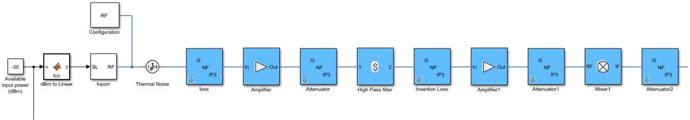
Image 38: Screenshot showing receiver chain exported to simulink environment (first half)
