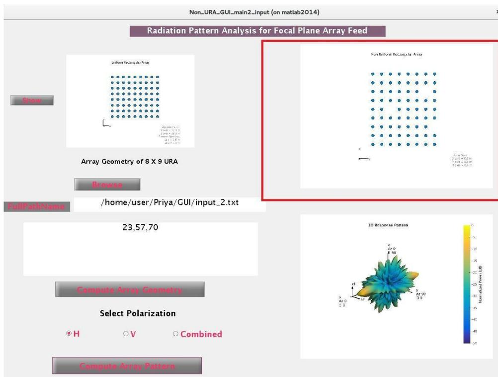
Image 43: Interface showing array geometry with removed elements
