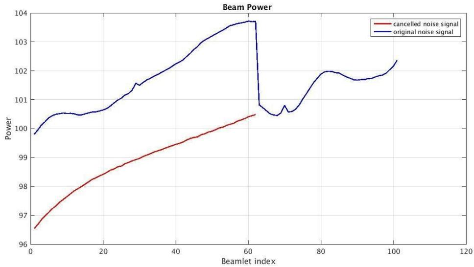
Image 17: Noise cancellation resulting 3dB change after applying the weights for 60 beamlets
