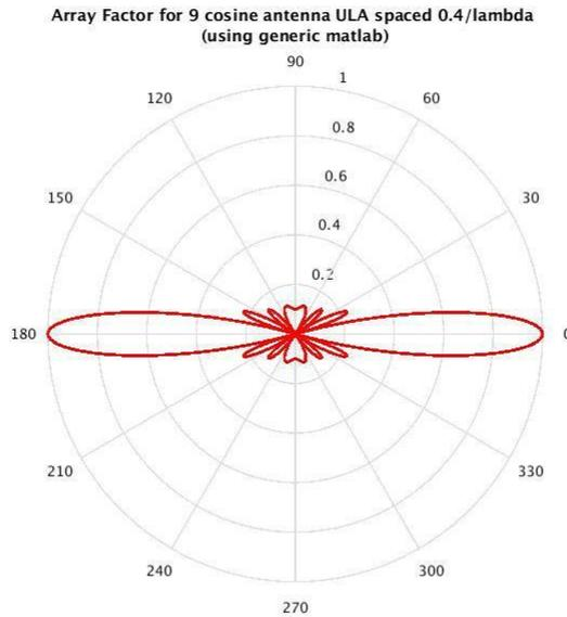
Image 29: Array factor for 9 cosine antenna ULA spaced  $0.4\lambda$
