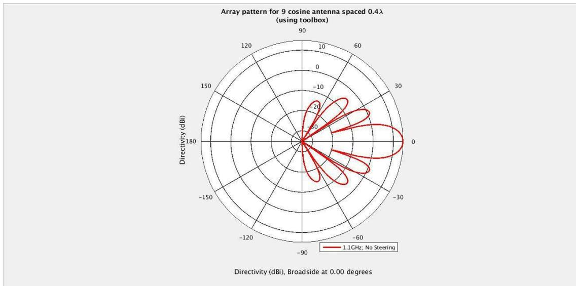
Image 31: Array directivity for 9 cosine antenna ULA spaced  $0.4\lambda$  using sensor array analyzer app
