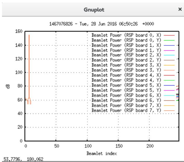
Image 10: Two tone signals added in phase (original amplitude 149 dB) after adding increased to 155 dB.
