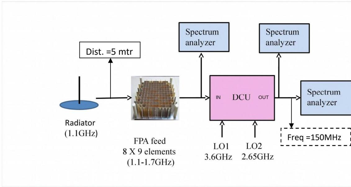
Figure 3: Experimental setup 2
