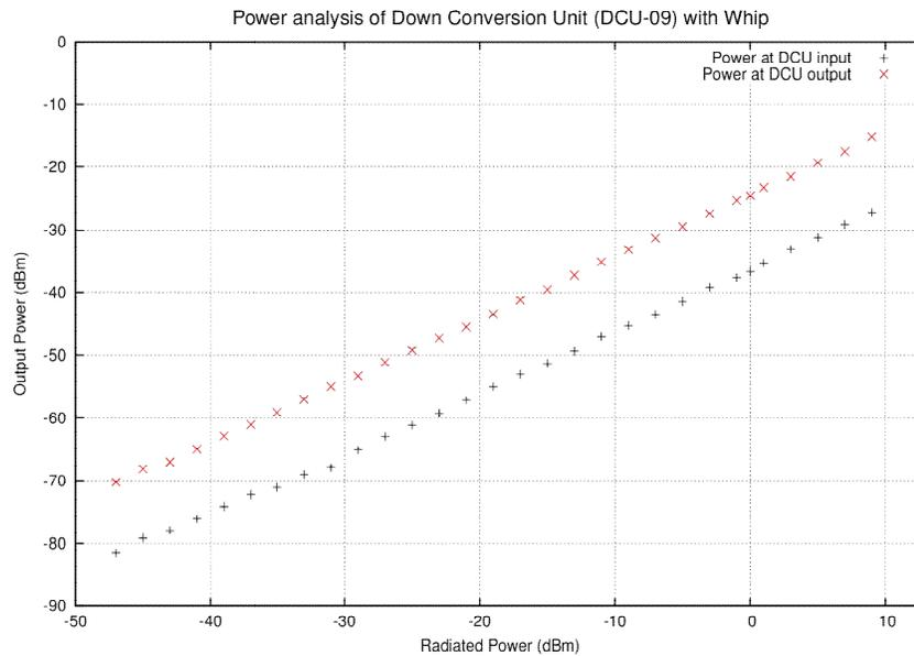
Image 15: Power analysis of DCU with whip antenna
