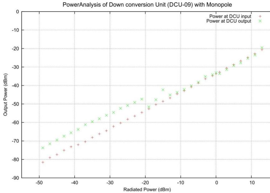
Image 14: Power analysis of DCU with monopole
