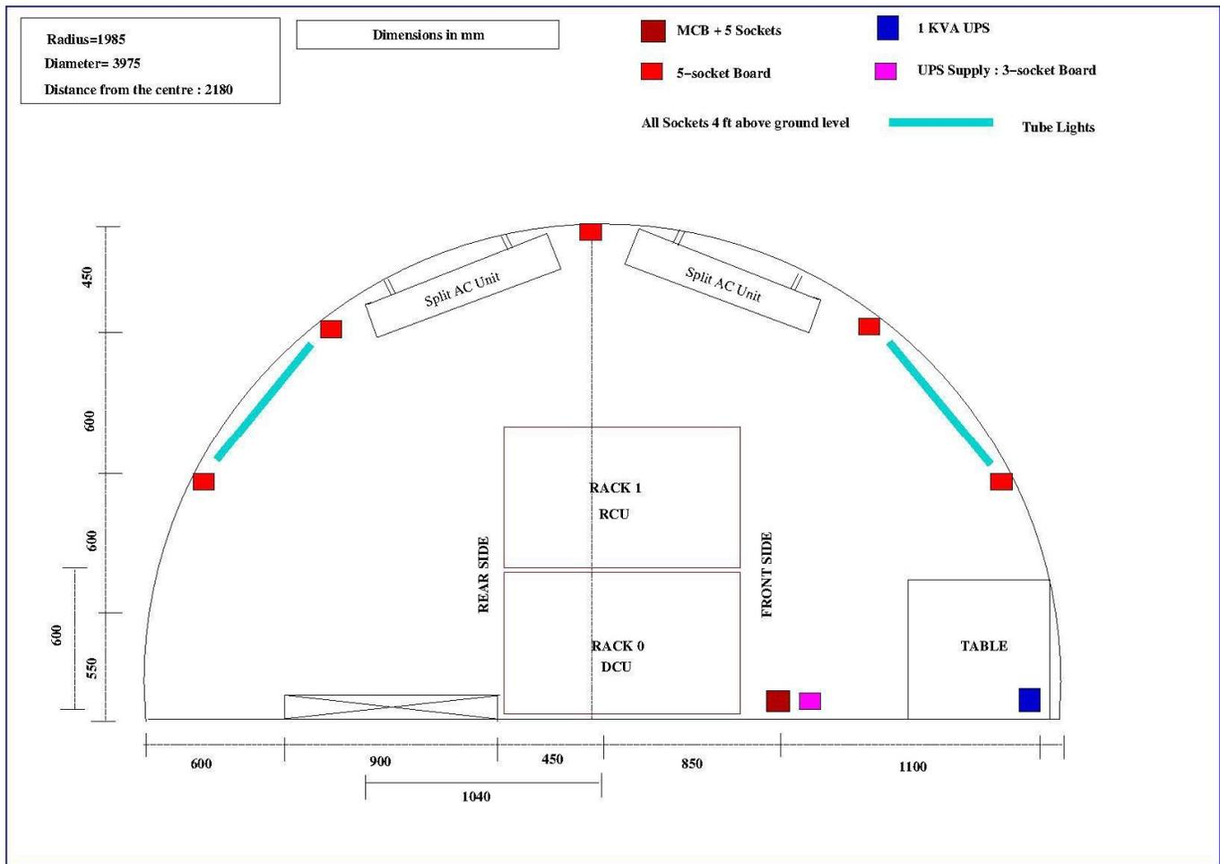
Image 18: Layout for arranging the FPA racks in glass room
