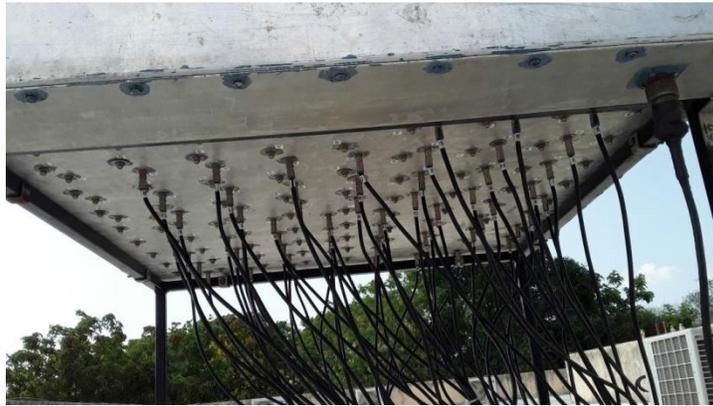
Image 6: Connecting 60 cables to the FPA feed and routing them
