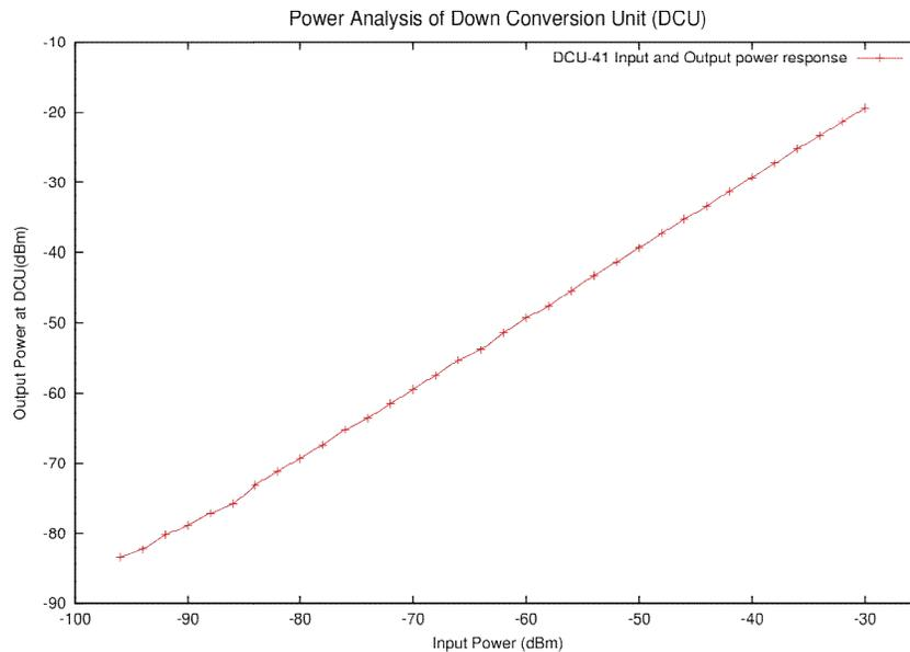
Image 13: Power analysis of Down Converter Unit
