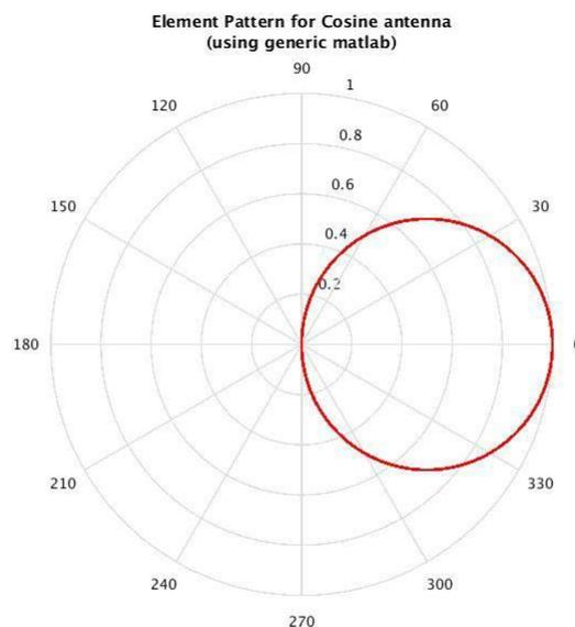
Image 28: Element Pattern for Cosine Antenna
