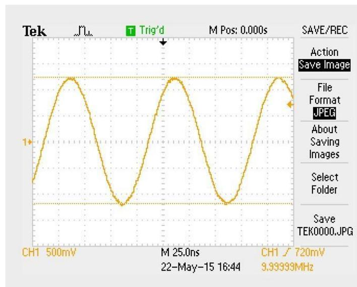
Image 4: Scope output plot for 10 MHz signal
