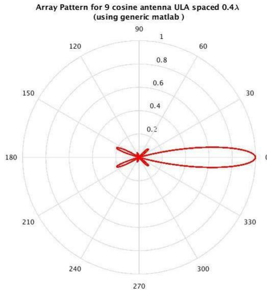
Image 30: Array Pattern for 9 cosine antenna ULA spaced  $0.4\lambda$
