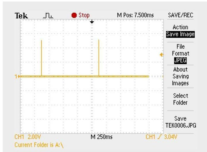
Image 5: Scope output plot for 1 PPS signal
