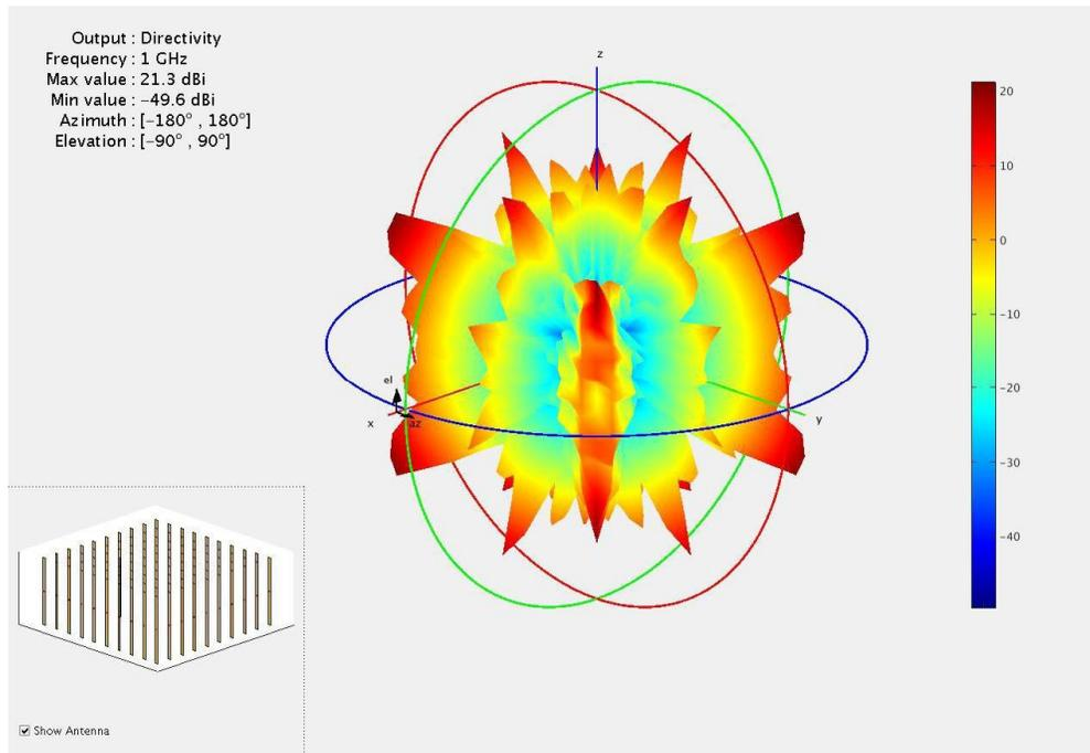
Image 27: Radiation pattern of uniform rectangular array
