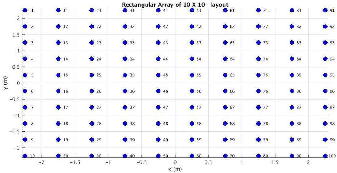
Image 25: Rectangular array layout for 10\*10 array of dipole antennas
