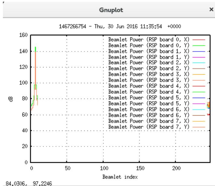
Image8: Twotonesignalsadded in phase with each other (original tone signal amplitude 139 dB) later increased to 145 dB
