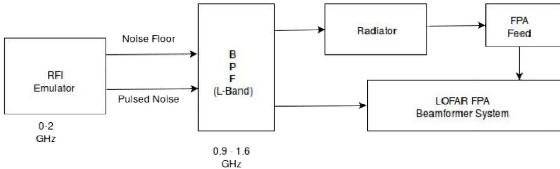
Figure 5: Test setup for noise test
