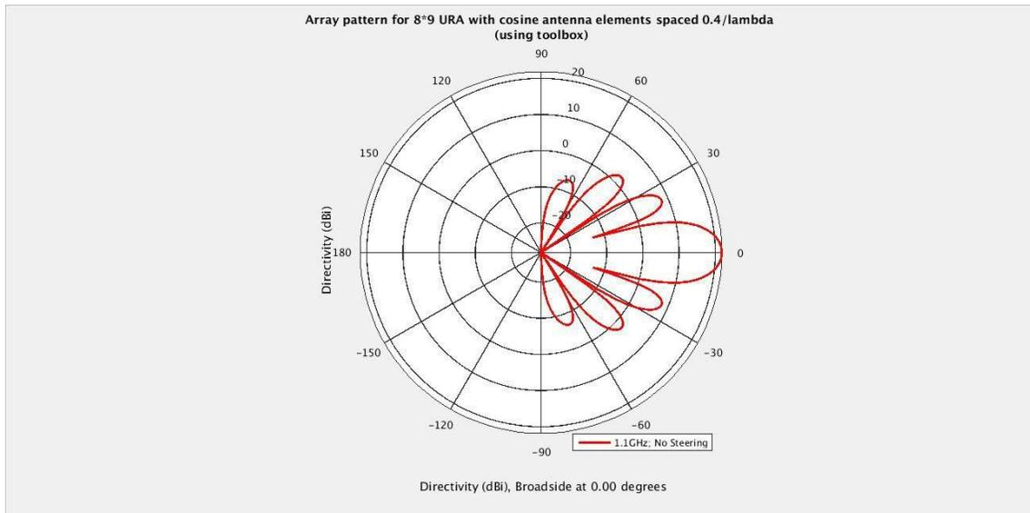
Image 32: Array directivity for 8\*9 array of cosine antenna URA spaced  $0.4\lambda$  using sensor array analyzer app.
