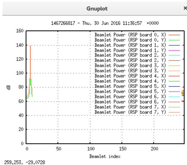
Image 9: Two tone signals provided out of phase (original amplitude 139 dB) later decreased to 133 dB.
